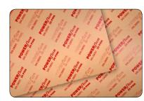
Structured PTFE - Gasket - Sheet manufactured by a unique process which provides a high level of fibrillation to overcome the creep relaxation and cold flow problem associated with normal (skived or moulded) PTFE sheets. POWER®flon 20 PINK is produced from virgin PTFE resin filled with Silica.
